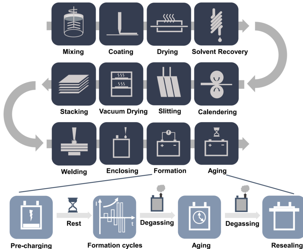
Figure 42: Schematic of lithium-ion battery manufacturing processes [132]
